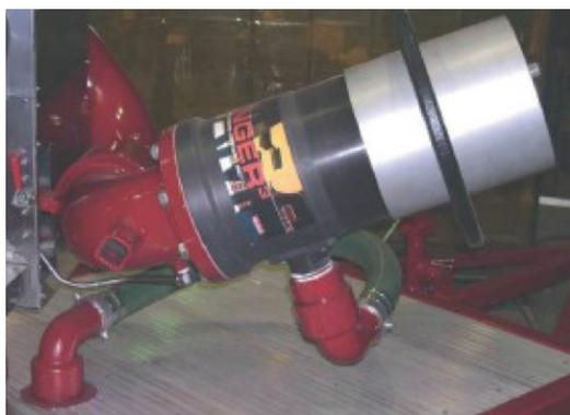
Esguicho Ranger3 da Willians. Vazão ajustável de 1000, 2000 e 3000 GPM. Alcance 100 PSI 30°: 1000 GPM: 75m, 2000 GPM: 100m e 3000 GPM: 110m.
